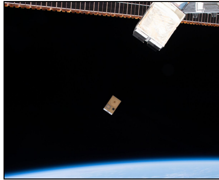
Figure 08. A photograph of a 2U CubeSat being deployed by the NanoRacks launch rails onboard the ISS [13].
